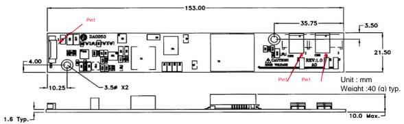
Note: Please use plastic screw in case of a non-insulating mounting base!
